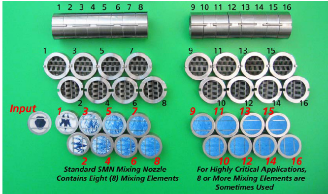
Fig. #3: Evolution of mixing through the SMN Static Mixer Elements with Blue and White resins (1:1 volumetric ratio). After 8 mixing elements, 80% and after 16 elements 97% of mixing efficiency is achieved.
