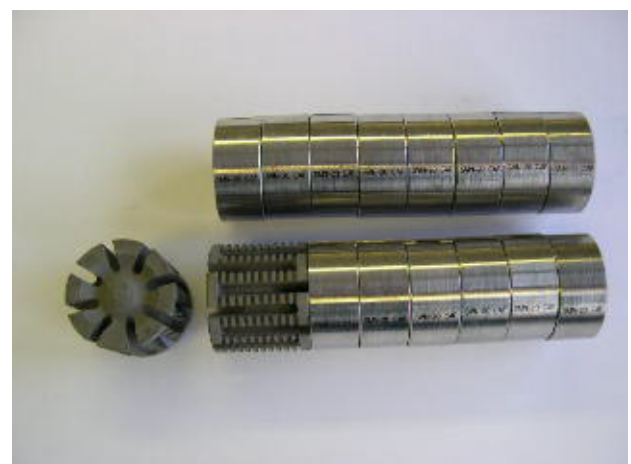
Eight (8) SMN mixing elements and six (6) elements combined with filter SMF.
