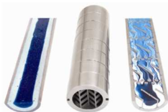
Fig. #1: Mixing of blue and white epoxy resins. Empty tube (left) provides no mixing. Eight (8) SMN mixing elements (center and right) provide an almost perfect mix.
